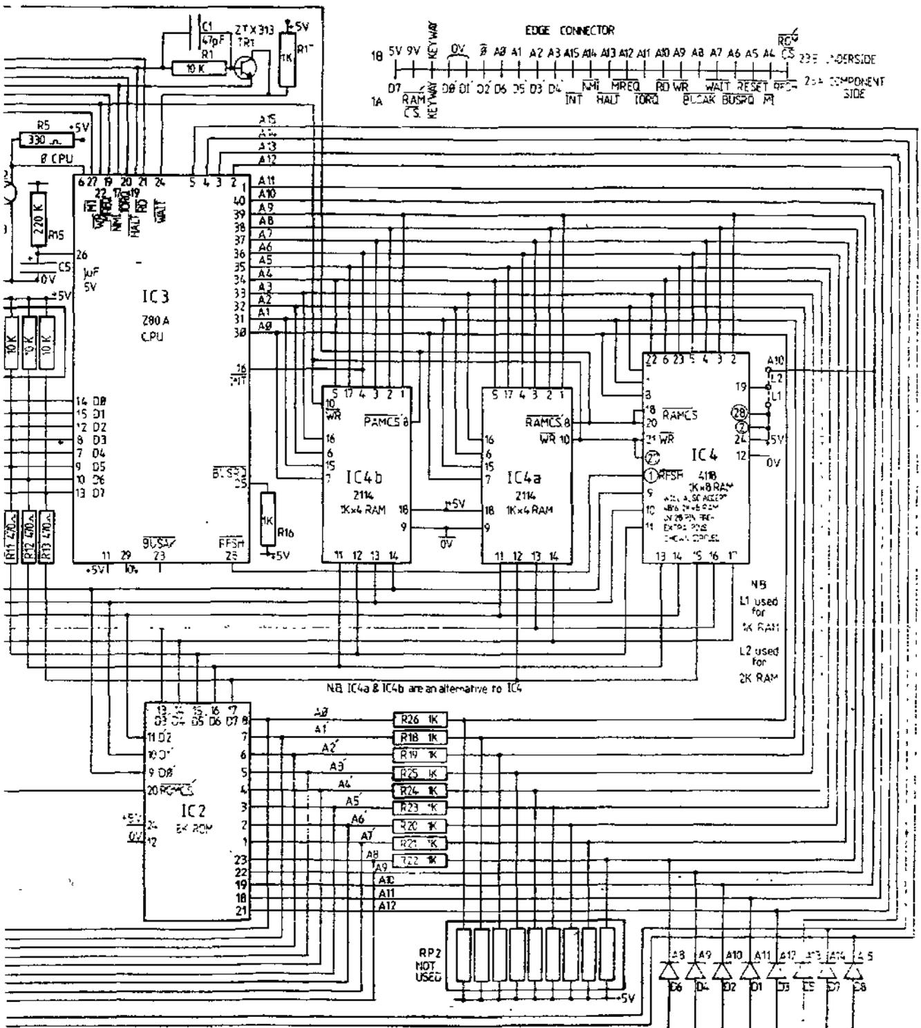
NB IC4a & IC4b are an alternative to IC4
