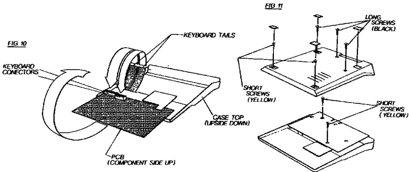
these locate Serious damage will result if the long screws are inserted in the wrong holes.
