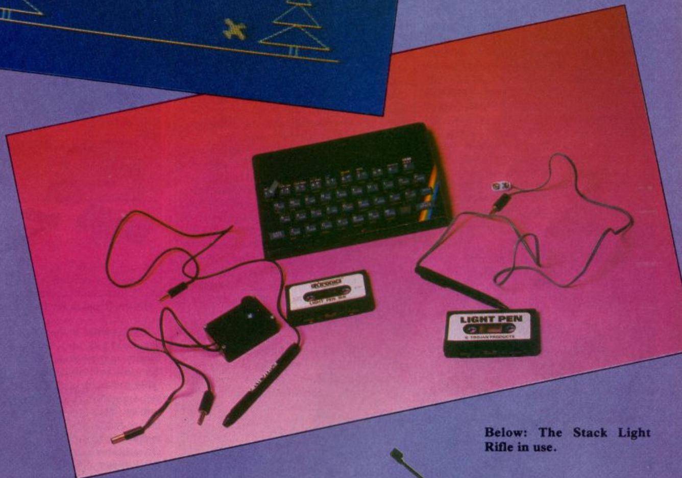
Below: Two Spectrum light pens, from dk'tronics and Trojan Products.
