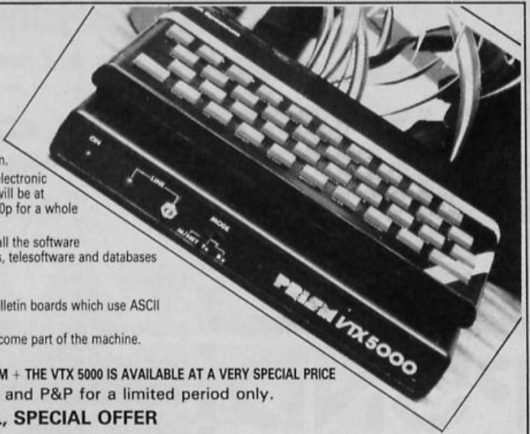
All modems provide 1200/75 baud, enabling access to Prestel, Micronet 800, BT Gold, Farmlink, Citiservices, Homelink, and some free bulletin boards (some databases and networks require a small subscription). Fully BT Approved.
