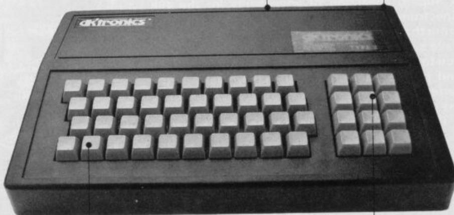
The legends for the keytops come as squares of printed sticky-back plastic that have to be stuck to the right keys DIY-style.
