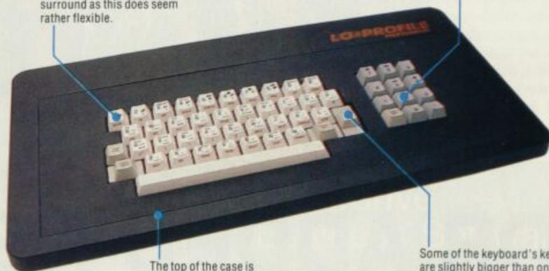
The cursor keys are repeated on the numeric keypad; also featured are a separate Caps Shift and '.' key as well.
