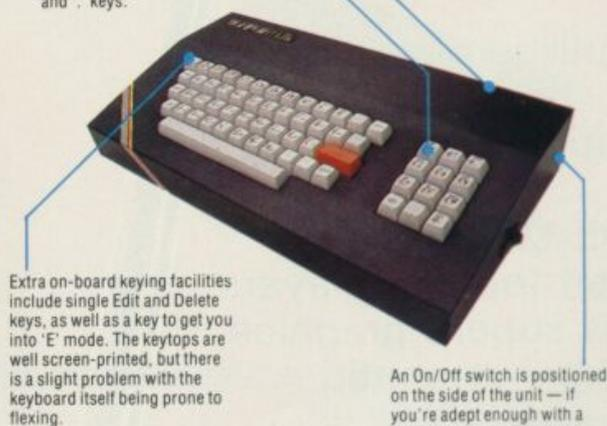
Extra on-board keying facilities include single Edit and Delete keys, as well as a key to get you into 'E' mode. The keytops are well screen-printed, but there is a slight problem with the keyboard itself being prone to flexing.
