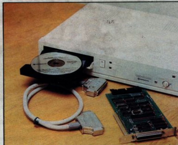
● The Hitachi 15035 is a CD-ROM optical disc drive with combined audio and stereo storage.
