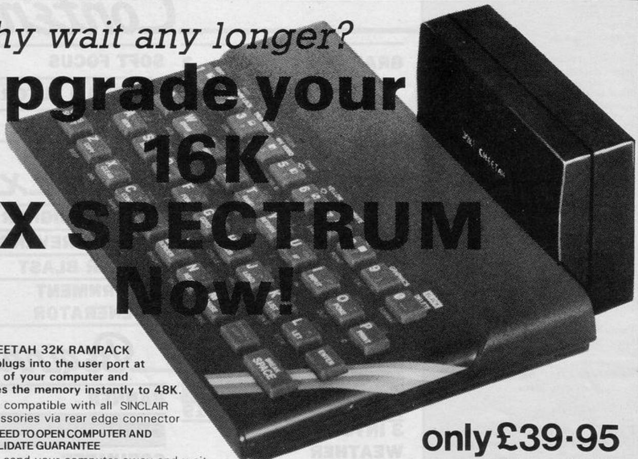
The CHEETAH 32K RAMPACK simply plugs into the user port at the rear of your computer and increases the memory instantly to 48K.
