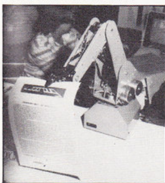
Colne Robotics' Armdroid showed off its five axes of rotation on the Laserbug stand.
