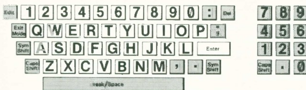
Fig. 3.3. Layout of the Transform keyboard.
