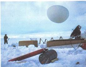
Unmanned weather balloons are used to record temperatures and air pressure high up in the atmosphere. Some send their readings back by radio signals, others are brought back to earth by radio control. The readings from these balloons help with weather forecasts.
