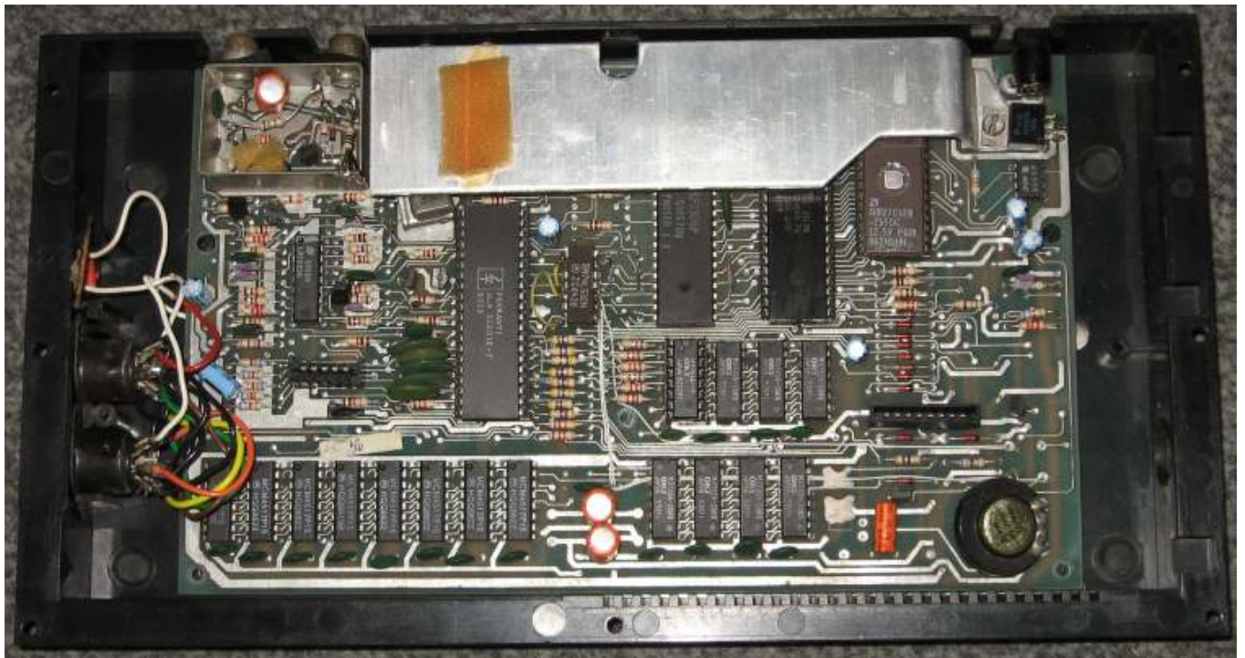
This is the Argentinean CZ Spectrum 48K, by Czerweny. The 8-pin DIN connectors are for Sinclair Joysticks; the red thing above is a reset button. Note the lack of coil for RAM power; it's been replaced with a NE555 as astable.
