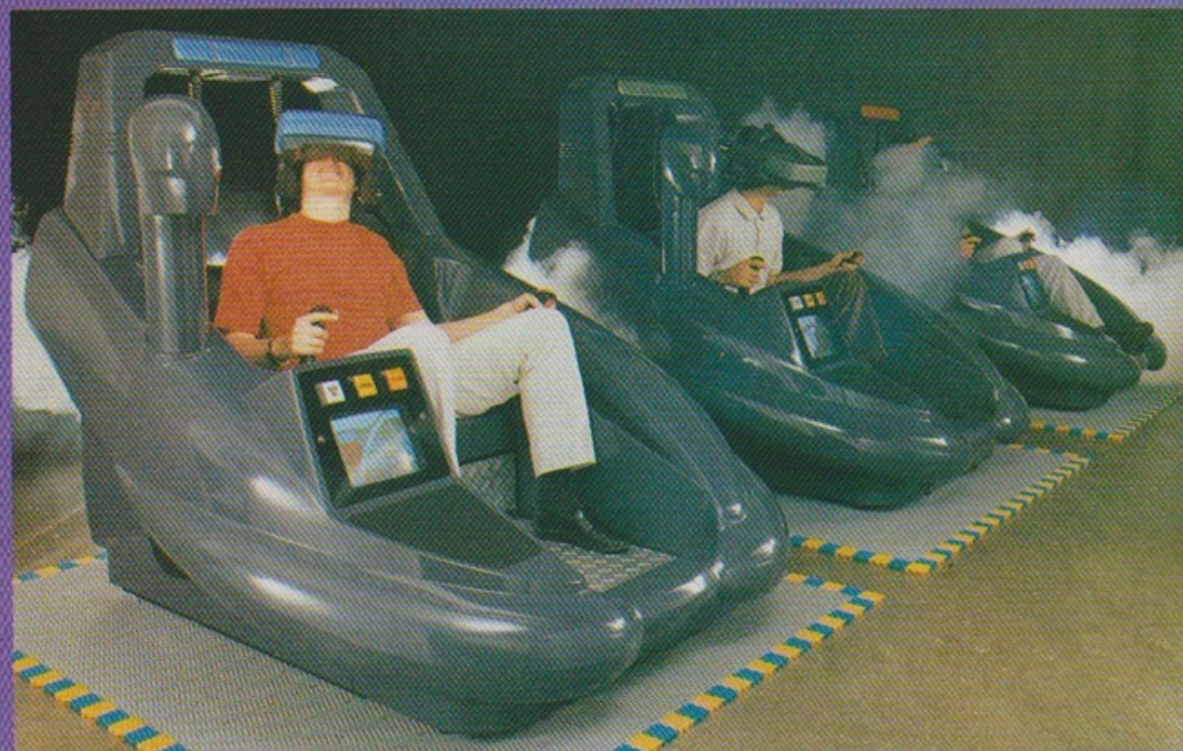
Virtuality 1000 SD, a high quality, 90-degree reclining seat which enables the operator to drive the 'vehicle' in a virtual world
