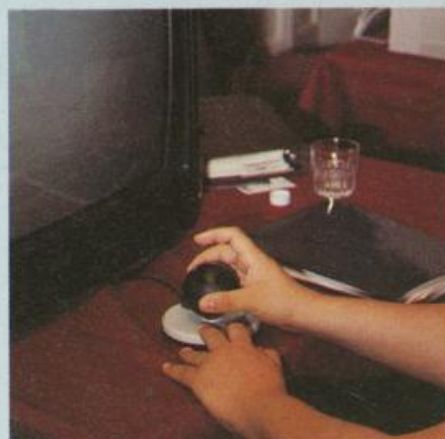
Using a GeoBall to control a screen display of a virtual world. The ball responds to pressure upwards and downwards, left and right, forward and backward, clockwise and anti-clockwise, giving 8D control – essential for manoeuvres in 3D space
