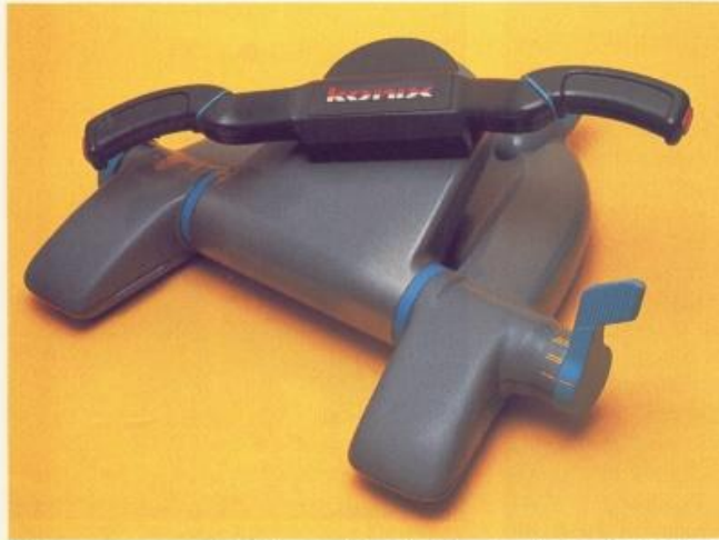
Vroom, vroom – motorbike mode. The two handgrips have been swivelled round, and the console stem locked in position.
