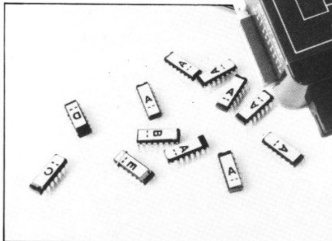
The 12 ICs which make the second issue 16K Spectrum up to a 48K device from JRS Software.
