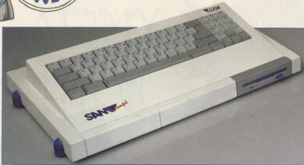
The Coupé's slot-in disk drive
