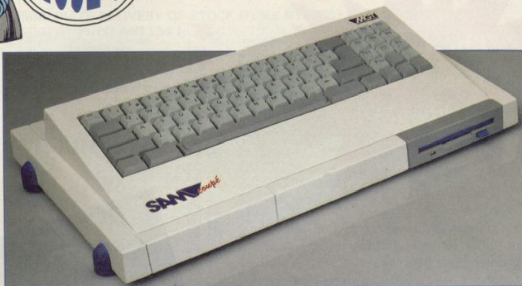
The Coupé's slot-in disk drive
