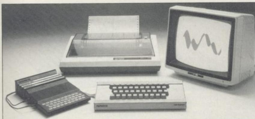
via a light-touch keyboard, construct and label graphs, and then copy the screen to an 80-column printer. Only 16K of memory is shown here but with additional memory, more than one video page can be stored. Up to 7 pages can be displayed in rapid succession to give animated displays.
