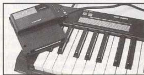
The FM sounds cover brass, piano, string, bass, metallic and abstract effects, providing much of the power and clarity of Yamaha's DX9 despite the use of only two sine wave operators. ◀
