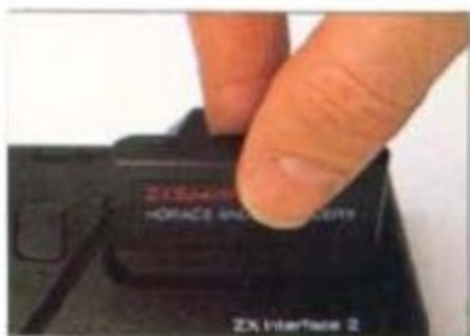
Plugging in a ROM cartridge The cartridge is inserted into the interface socket. When the computer is powered up, the program is automatically loaded, bypassing the ROM inside the computer.
