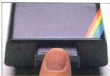
Loading a Microdrive Microdrive cartridges are inserted into the slot in front of the drive.
